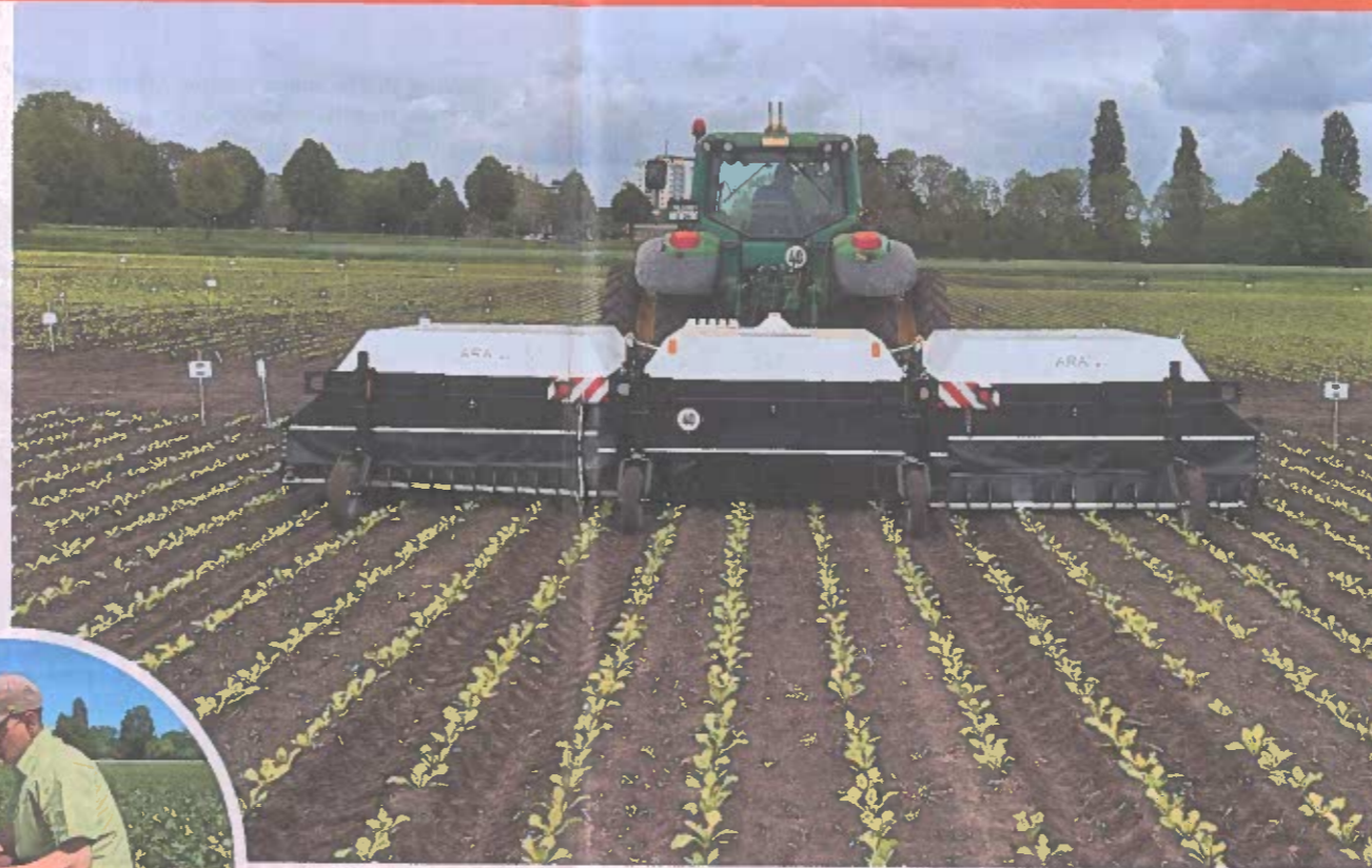
The Ecorobotix ARA spot sprayer can cover up to 4ha an hour
